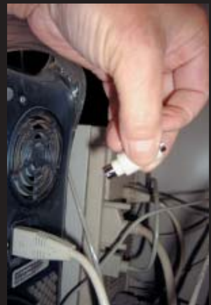
Installing a KeyKatcher bug on a computer takes seconds
